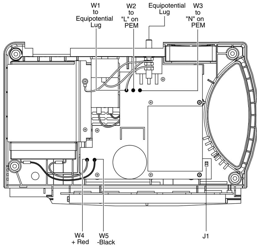
**Figure 6-5: Internal Power Connections**
