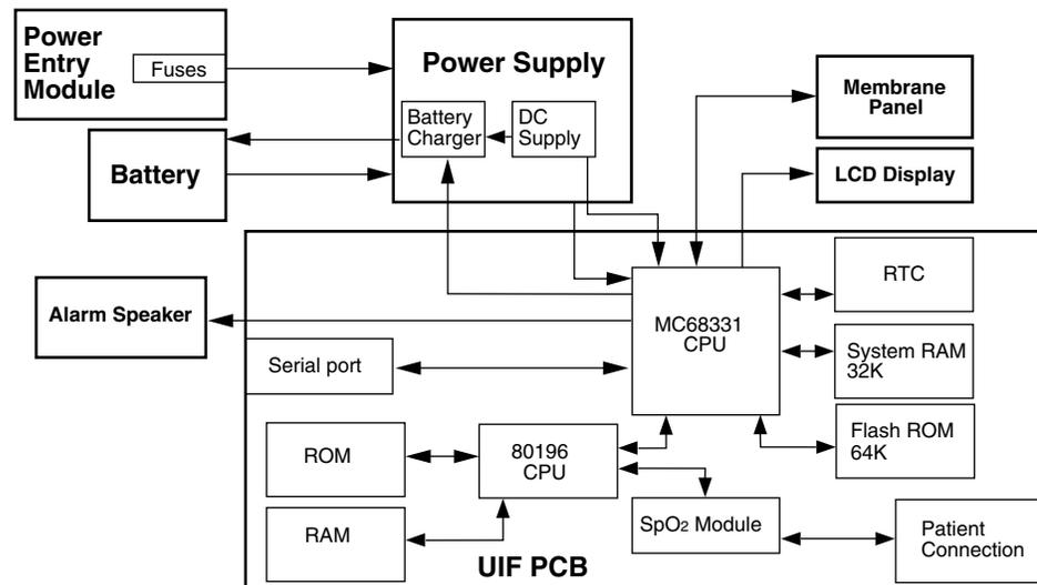
Figure 11-2: NPB-195 Functional Block Diagram
